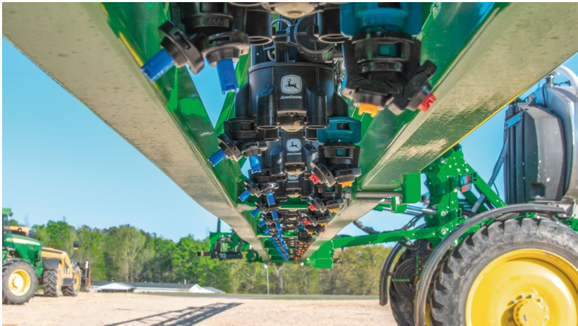
Blended Pulse™ DualFan BPDF06 nozzles field testing on a John Deere ExactApply™ PWM equipped sprayer in Mississippi
