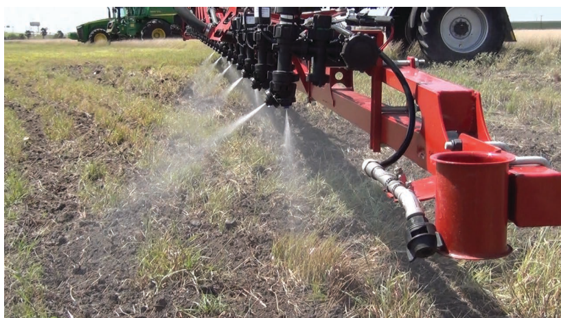
SprayMax DualFan DF20 nozzles running on an Aim Command™ PWM equipped sprayer at a Greenleaf Technologies dealer in Texas
